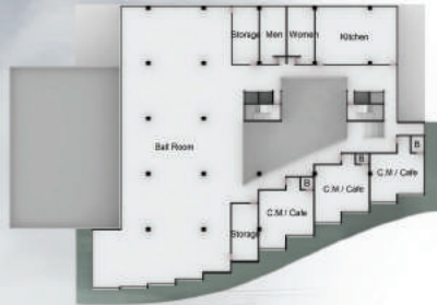
2nd Floor Plan Scale: 1:300
